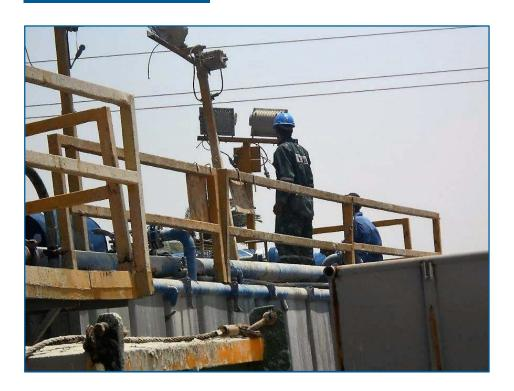
The dry location technology is a new approach for waste management. Dry location technique is used to eliminate the waste pit and reduces the drilling fluid (Water Base Mud or Oil Base Mud) on cuttings to below 10% instead of 40%. Moreover, the drilling fluid and cutting are separated into two main streams. Liquid (liquid waste water) and semi dry (drilling cutting or drilling mud cuttings). Waste pits are replaced with tank, 10 tons box for the solid waste and 500 bbl for the liquid waste.
